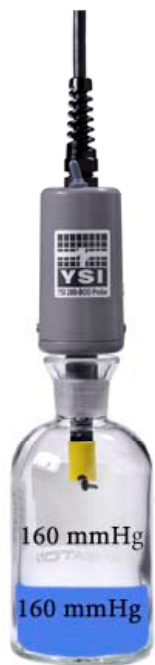
Figure 37. The oxygen pressure in water-saturated air and air-saturated water is 160 mmHg at sea level.
