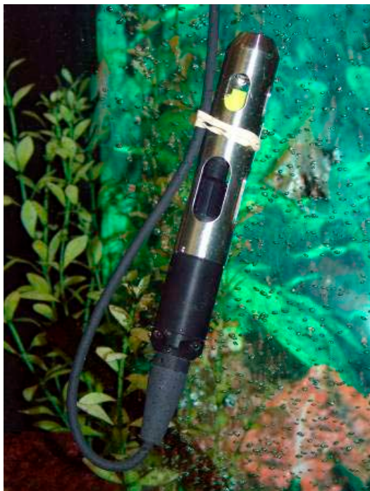
Figure 39. DO sensor inverted to avoid air bubbles bursting on the membrane surface.
