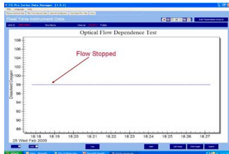
Figure 28. A graph, created in YSI Data Manager software program, illustrating the flow independence of an optical sensor.
