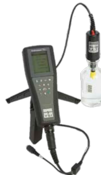
Figure 11. The Professional Plus multiparameter instrument with a BOD-style sensor. The Professional Plus can be outfitted with several different single and multi-parameter cables including the Quatro which can measure dissolved oxygen, temperature, conductivity, and two ISEs at the same time and on the same cable.
