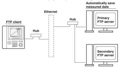
You can specify two destination FTP servers, primary and secondary. If the primary server is down, the file is transferred to the secondary server.
