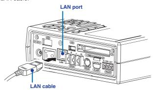
If you are connecting the XL100 and the PC directly in a one-to-one configuration without using a hub, use a cross LAN cable.
