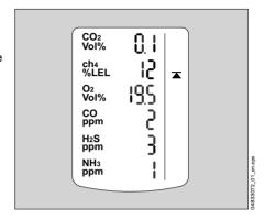
The peak values can be deleted by pressing the key for 5 sec. The adjacent display appears.
