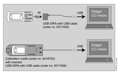
The installed PC software Dräger CC Vision is used for configuration.
