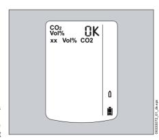
Close the test gas cylinder valve and remove the instrument from the calibration cradle.
