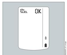
Close the test gas cylinder valve and remove the instrument from the calibration cradle.
