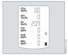
button calibration will be aborted. The channels will then indicate \* n/a \*. If only one sensor is taking part in the 1-button calibration, a calibration will be performed in each case when the (\* key is pressed.
