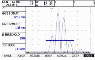
measured sound path: 12.35 mm amplitude: 37 %
