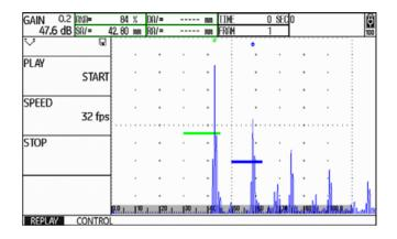
The control functions in the function groups **REPLAY** and **CONTROL** are displayed next to the A-scan.
