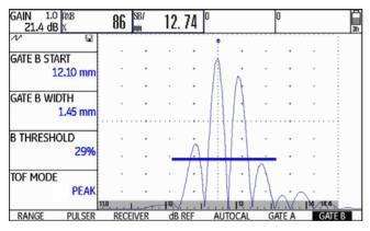
measured sound path: 12.74 mm amplitude: 86 %
