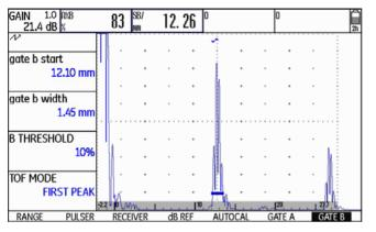
measured sound path: 12.26 mm amplitude: 83 %
