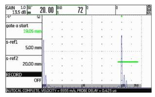
You can read the material velocity and the probe delay in the function group **RANGE**.
