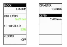
In this regard, it is important that **DEPTH** always refers to the center of the side-drilled hole and not to the real reflecting surface.
