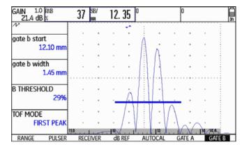
measured sound path: 12.35 mm amplitude: 37 %
