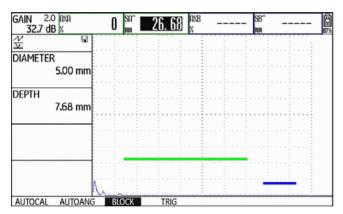
The side-drilled hole is located at a depth of 7.68 mm and has a diameter of 5.00 mm.
