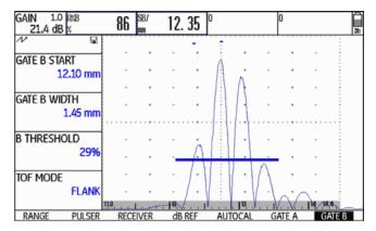
measured sound path: 12.35 mm amplitude: 86 %
