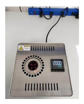
The Blackbody insert fits into the heater block just like the standard inserts using the insert extractor tool. The target source is 1.3" in diameter.
