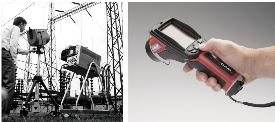
Figure 22.1 LEFT: Thermovision® Model 661 from 1969. The camera weighed approximately 25 kg (55 lb.), the oscilloscope 20 kg (44 lb.), and the tripod 15 kg (33 lb.). The operator also needed a 220 VAC generator set, and a 10 L (2.6 US gallon) jar with liquid nitrogen. To the left of the oscilloscope the Polaroid attachment (6 kg/13 lb.) can be seen. RIGHT: InfraCAM from 2006. Weight: 0.55 kg (1.21 lb.), including the battery
