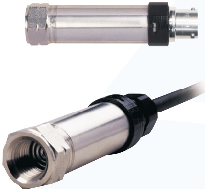
The SPX 2000 Series pressure sensors are designed using field-proven piezoresistive silicon technology, coupled with advanced ASIC electronic compensation techniques, that result in a true, high-performance, low-cost family of products. The use of NACE-compatible 316L SS and Hastelloy wetted parts ensure material compatibility in harsh environments. The modular construction is well suited for customization for OEM, reseller, and large end-user applications.
