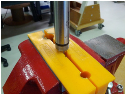
Cabled Sensor—gripping on swage
