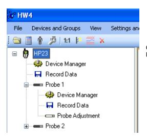
Click on the + sign to the left of a probe icon to display a list of the available functional modules for the probe.
