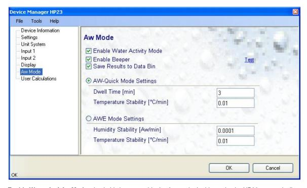
**Enable Water Activity Mode**: check this box to enable the Aw mode. In this mode, the HP23 automatically displays humidity as  $a_w$  (1.00  $a_w$  = 100 %RH)
