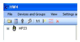
After detection by HW4, the HP23 appears as an icon in the left pane of the HW4 main screen.
