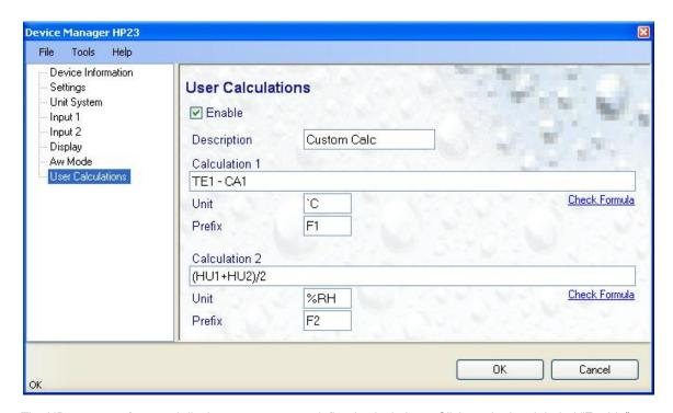
The HP23 can perform and display up to two user defined calculations. Click on the box labeled "Enable" to turn on this function. A check mark appears.
