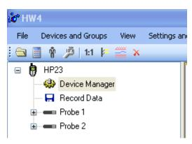
To select the Device Manager for the HP23, click on it with the left mouse button. HW4 opens the Device Manager form.
