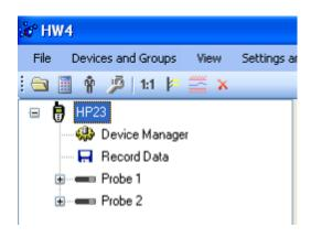
Click on the + sign to the left of the HP23 icon to display the HP23 Device Manager module, the Record Data module as well as two probe icons (one for each of the HP23 inputs).
