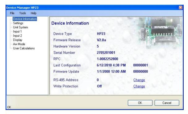
**RS485 Address**: click on the underlined blue link to change the transmitter address to be used in conjunction with an RS-485 network (multi-drop). Each network address should be unique and within the values of 1 to 64. Note: the default factory RS-485 address is 0. Click on the Device Manager OK button to write the new address to the transmitter.
