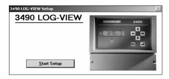
If <u>Start Setup</u> is chosen (Figure 1), the screen will then ask where the program is to be installed. The default location of "C:\ LOGVIEW" will be displayed. If a different path is required, edit the "Install To:" text box (Figure 2).
