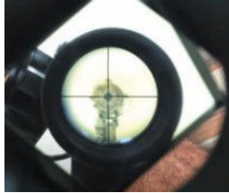
Figure 5-7: View through the Alignment Tool
