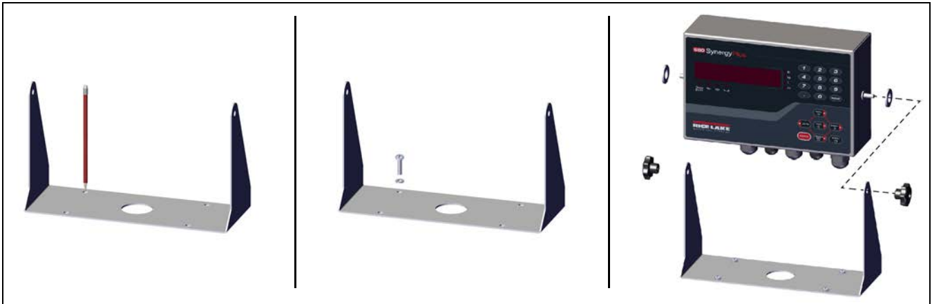
Figure 2-3. Mounting the Indicator
