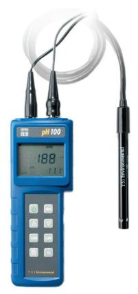
The pH100 with one of the possible configurations using a combination 2-in-1 pH sensor and temperature sensor. Another option allows for a mV or pH sensor with a separate temperature sensor or flat tipped and piercing tipped probes.
