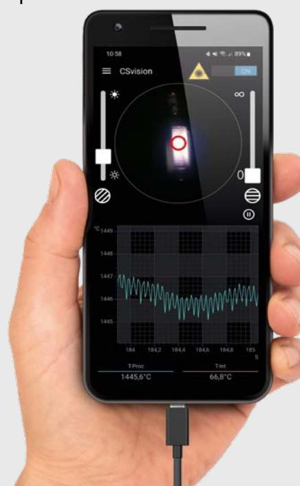
The innovative two-step brightness reduction filter uncovers tiny details: here of a filament.
