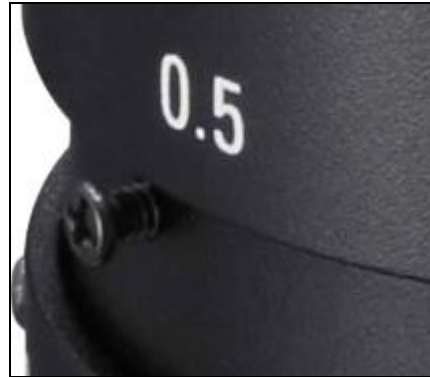
Figure 18: Fixing the focus for PI 05M/ 08M/ 1M
