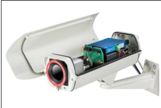
Figure 29: Outdoor protective housing for PI camera, USB server and industrial PIF
