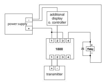
Separate power supply for measurement section and output section
