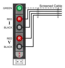
The screen should also be connected to the outer sheath of the PRT (if it is metal clad). The use of screened cables is more important when the milliK is used with thermistors, which have a higher resistance than PRTs or thermocouples.
