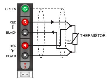
Because the resistance of thermistors used for temperature measurement is much higher than for PRTs, lead resistance is not normally a problem.
