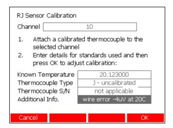
Press the OK (F4) key to start the calibration adjustment. Once started, the calibration adjustment process cannot be aborted.
