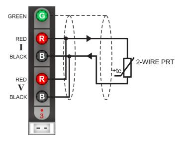
The connections to the PRT should be short (low resistance) in order to minimise the effect of lead resistance on the measurement. Alternatively, the connections can use remote sensing (using the 4-wire measurement capability of the millik) to eliminate the effect of lead resistance completely. In this arrangement, the current and voltage sense connections are kept separate and are only joined close to the PRT:
