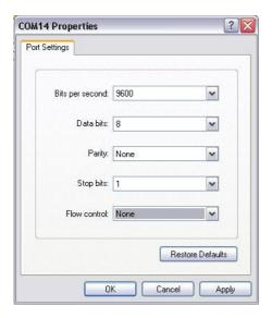
Click OK to open a Hyperterminal session with the millisKanner. Type \*/DN? into Hyperterminal (terminate the command by pressing the carriage return or Enter keys), the millisKanner should then respond with a string in the form:
