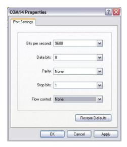
Click OK to open a Hyperterminal session with the millisKanner. Now save (using File|Save As) the Hyperterminal connection so that in future you only have to click on this icon to open an RS232 connection with your millisKanner.
