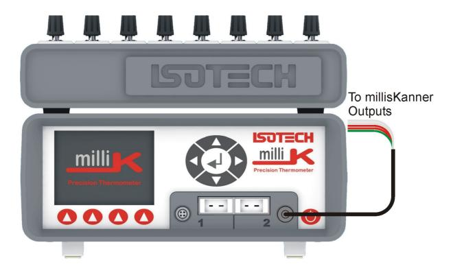
Note the scanner output must be connected to Channel 2 of the milliK
