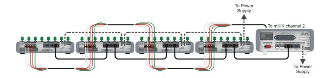
If you wish to make your own analogue link cables, use a screened cable with low dielectric loss insulation such as PTFE or polyethylene (otherwise measurement performance may be affected). The screen should be connected to the ground terminals on both millisKanners.
