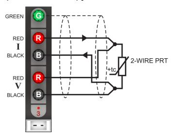
The top (green) terminal should be connected to the screen of the PRT's lead (where present) to minimise electrical noise picked up by the wires.
