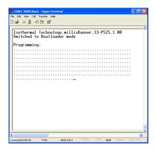
When the firmware update is complete the millisKanner will report "programming successful – jumping to loaded application". Now send \*/DN? to confirm that the millisKanner firmware is loaded and running:
