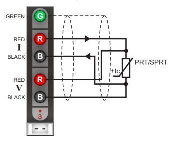
The top (green) terminal should be connected to the screen of the PRT's lead (where present) to minimise electrical noise picked up by the wires.
