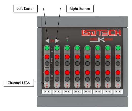
The millisKanner starts up with no channel selected. Pressing the 'Right' button will then select Channel 0. Press the 'Right' button when Channel 7 is selected or the 'Left' button when Channel 0 is selected to turn off all channels. The 'Channel LEDs' indicate which channel is selected.
