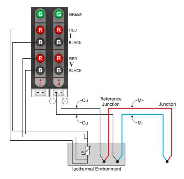
This technique is less accurate than using an ice-point due to the additional uncertainties associated with the PRT or thermistor used to monitor the reference junction and any temperature gradients between the temperature of the PRT/thermistor and the thermocouple's reference junction.
