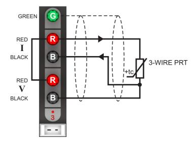
The connection between the positive (red) terminals should carry no current and should be connected as close to the base of the I+ terminal as possible in order for the 3-wire compensation to work effectively. The lowest 3-wire compensation error is achieved by using a wire under the screw terminal to connect the positive terminal together and then adding the 'single' PRT lead to the binding post:
