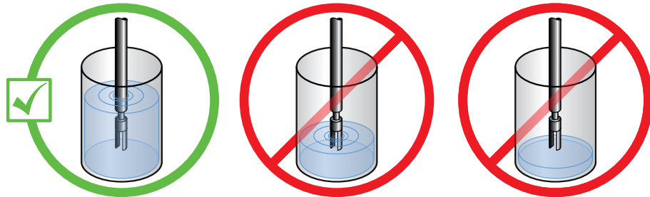
Figure 3-14: Meter placement (immersed in fluid)
