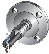
Figure 3-5: Free-stream (weldolet fitting) meter installation
