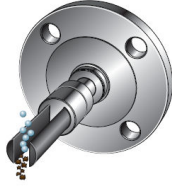
Figure 3-1: Free-stream flanged fitting meter installation
