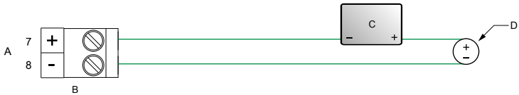
Figure 3-24: mA input wiring (externally powered)
