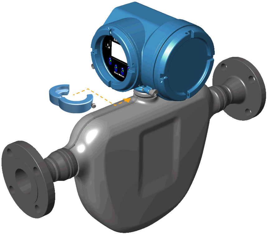
Figure 2-11: Re-attachment of the sensor clamp
