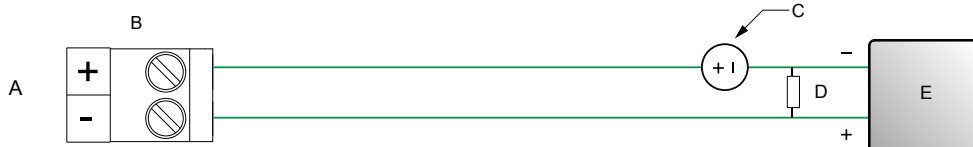
Figure 3-2: Externally-powered mA Output wiring
