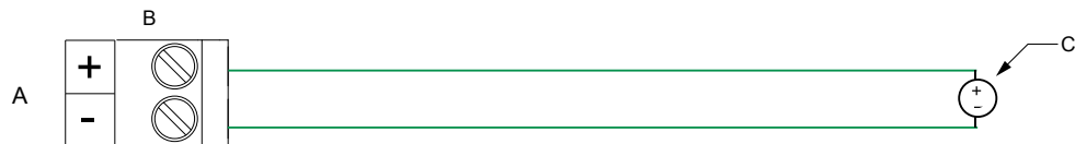
Figure 3-11: Externally-powered DI wiring
