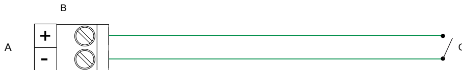
Figure 3-10: Internally-powered DI wiring
