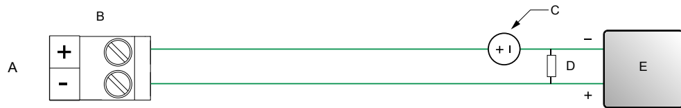
Figure 3-6: Externally-powered FO wiring
