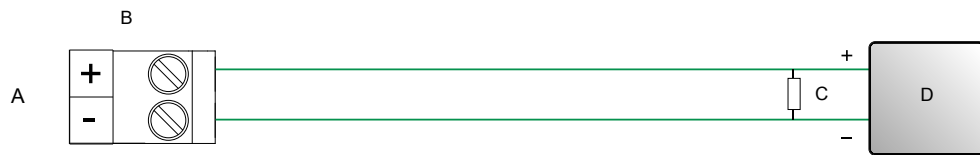
Figure 3-4: Internally-powered FO wiring
