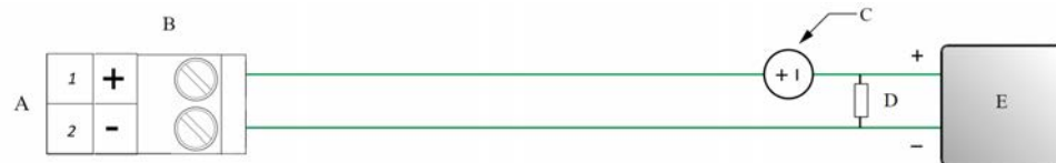
Figure 3-13: Frequency output wiring (externally powered)
