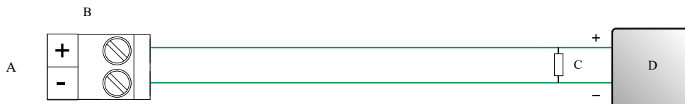
Figure 3-17: Discrete output wiring (internally powered)
