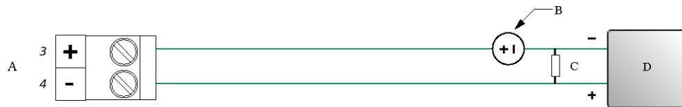
Figure 3-16: Frequency output wiring (externally powered)
