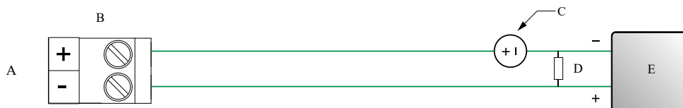
Figure 3-19: Discrete output wiring (externally powered)
