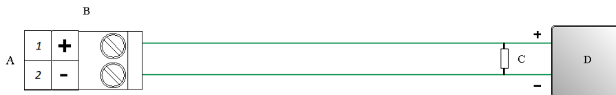
Figure 3-11: Frequency output wiring (internally powered)
