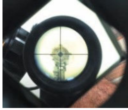
Figure 5-7: View through the Alignment Tool
