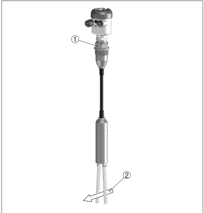
Fig. 6: Orientation of the tuning fork in case of flow
