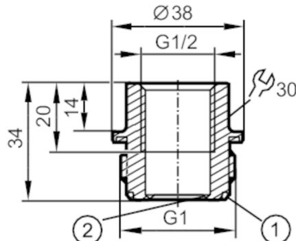
1 Sealing Aseptoflex Vario adapter
