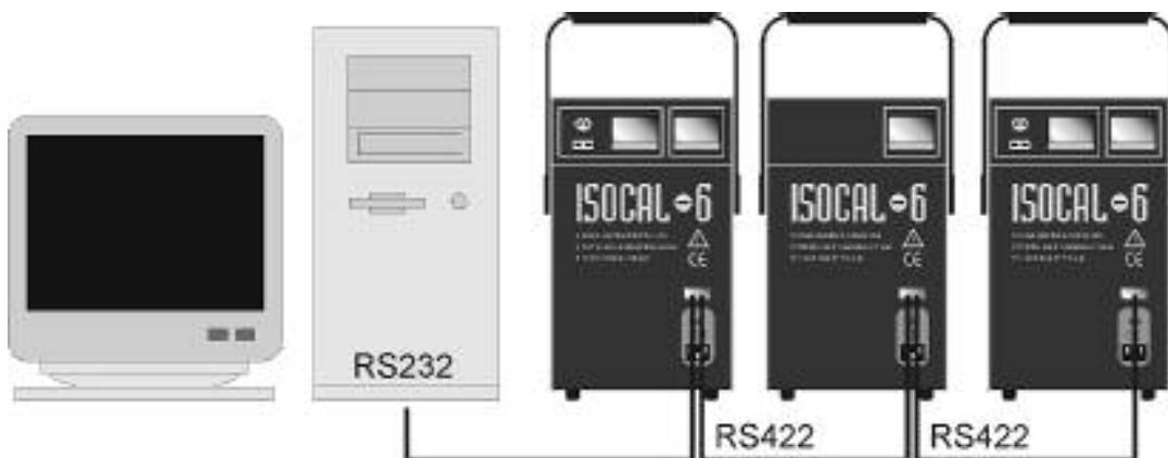
Note: The RS 422 standard specifies a maximum lead length of 1200M (4000ft). A true RS422 port will be required to realise such lead lengths. The Isotech conversion leads are suitable for maximum combined lead lengths of 10M that is adequate for most applications.
