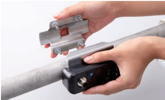
Clamp-on type without pipe modification.
