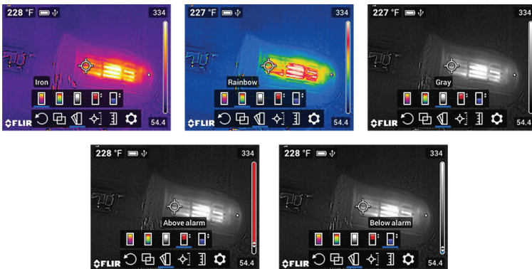
Figure 7.7 Selecting a Color palette or an Isotherm Alarm (Above and Below) mode.
