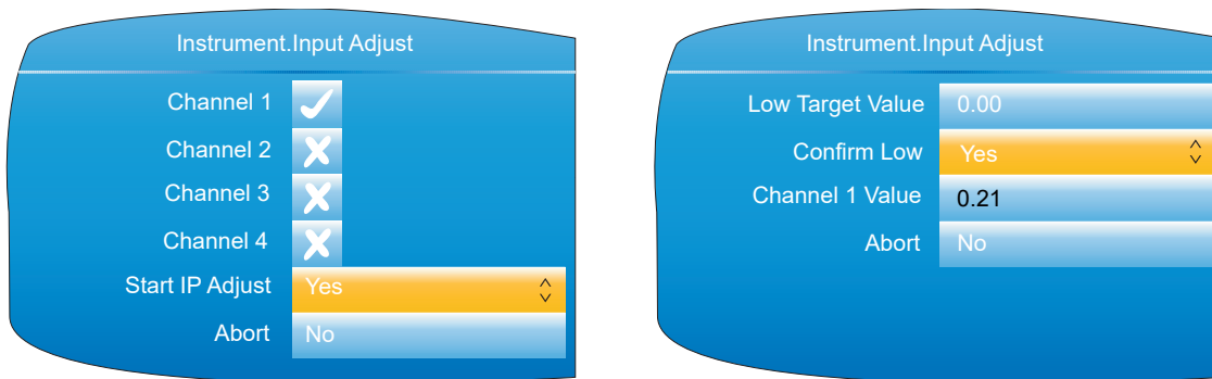
Figure 73 Channel adjustment procedure (2)
