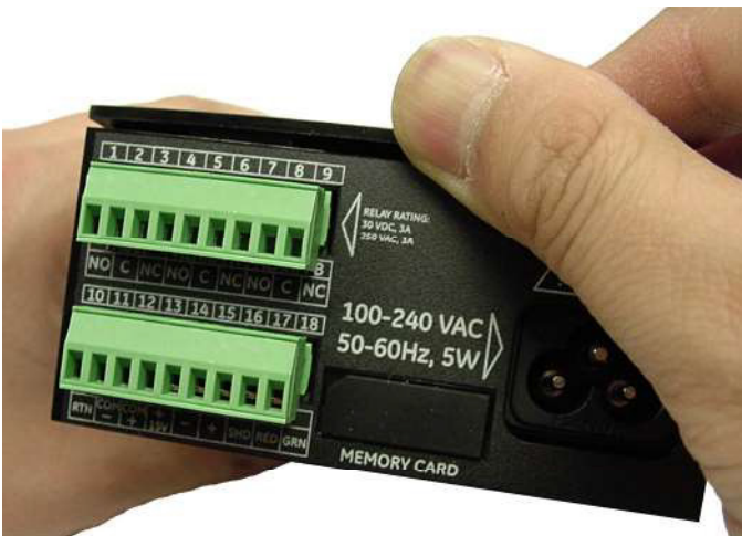
Figure 5: Lifting the Back Edge of the Cover
