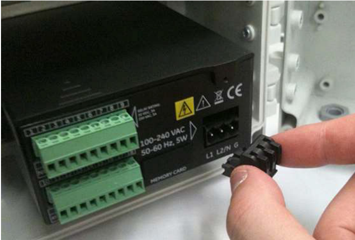
Figure 35: Removing the AC Power Connector
