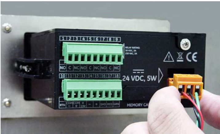
Figure 34: Reinserting the DC Power Connector
