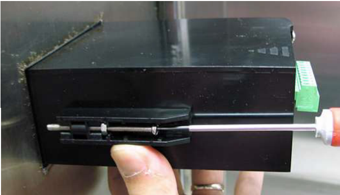
Figure 14: Securing the dew.IQ to the Panel
