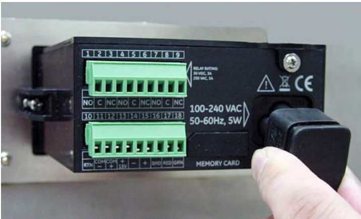
Figure 31: Inserting the AC Power Cable
