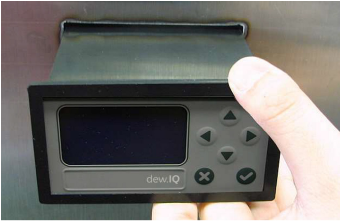
Figure 11: Sliding the dew.IQ into the Panel Cutout
