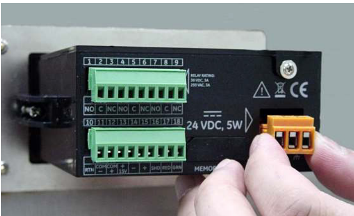
Figure 33: Removing the DC Power Connector
