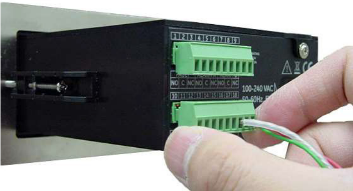
Figure 25: Reinserting the Connector into the Terminal Block
