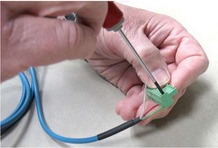
Figure 24: Making Probe Cable Connections to the Connector
