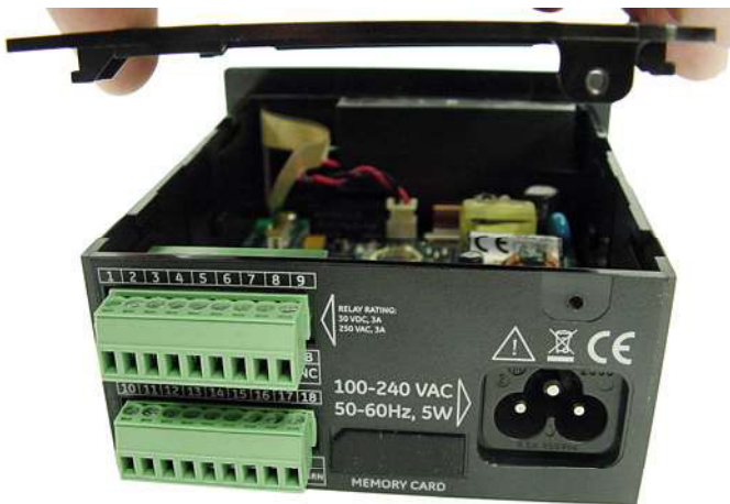
Figure 7: Removing the Cover
