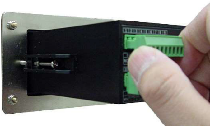
Figure 30: Removing the Upper Connector
