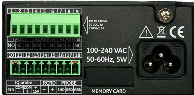
Figure 27: Bottom Connector Removed
