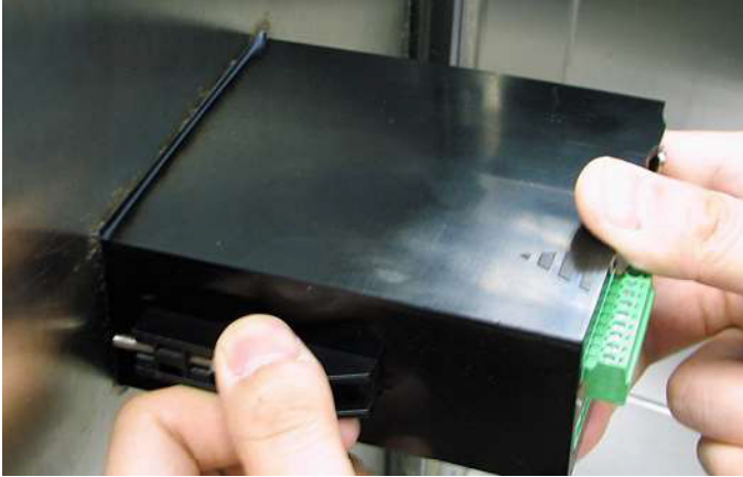
Figure 13: Locking the Mounting Brackets in Place
