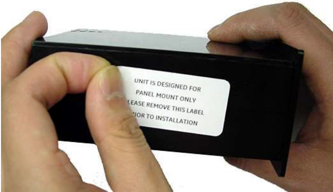
Figure 9: Removing Side Panel Mount Label
