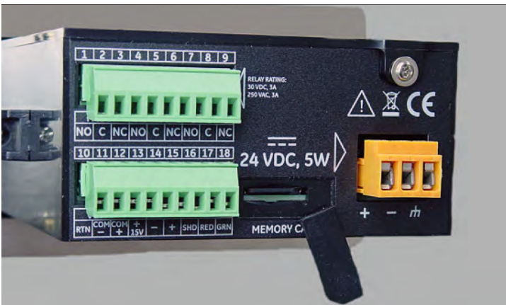
Figure 49: The Exposed Memory Card Holder
