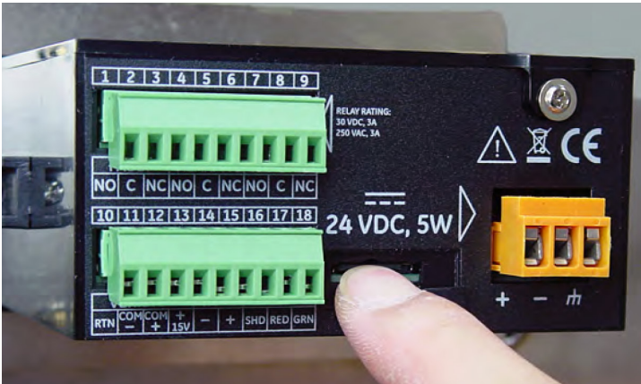
Figure 50: Pushing in on the MicroSD Card
