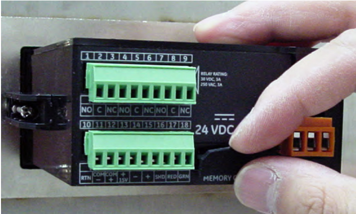
Figure 48: Pulling the Flexible Cover
