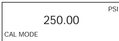
Use the Pressure Standard to output 250.00 psi (50%). After the output has stabilized, press the ENTER key to continue. As the unit takes readings, the screen will show \_\_\_\_\_. When the readings are complete the screen should look as shown below.
