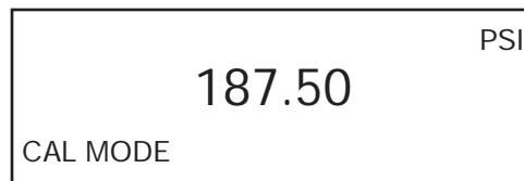
Use the Pressure Standard to output 187.50 psi (37.5%). After the output has stabilized, press the ENTER key to continue. As the unit takes readings, the screen will show \_\_\_\_\_. When the readings are complete the screen should look as shown below.
