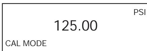
Use the Pressure Standard to output 125.00 psi (25%). After the output has stabilized, press the ENTER key to continue. As the unit takes readings, the screen will show \_\_\_\_\_. When the readings are complete the screen should look as shown below.
