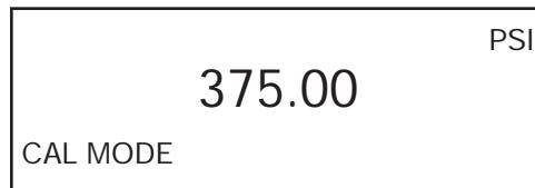
Use the Pressure Standard to output 375.00 psi (75%). After the output has stabilized, press the ENTER key to continue. As the unit takes readings, the screen will show \_\_\_\_\_. When the readings are complete the screen should look as shown below.
