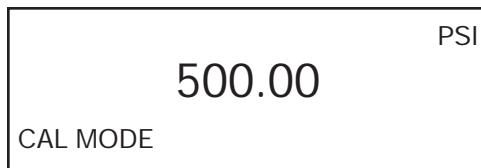
Use the Pressure Standard to output 500.00 psi (100%). After the output has stabilized, press the ENTER key to continue. As the unit takes readings, the screen will show \_\_\_\_\_. When the readings are complete the screen should look as shown in the illustration that follows.
