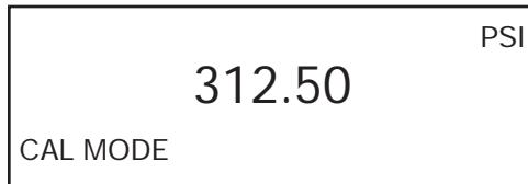
Use the Pressure Standard to output 312.50 psi (62.5%). After the output has stabilized, press the ENTER key to continue. As the unit takes readings, the screen will show \_\_\_\_\_. When the readings are complete the screen should look as shown below.
