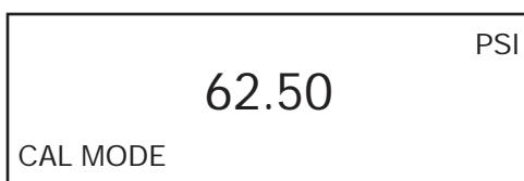
Use the Pressure Standard to output 62.50 psi (12.5%). After the output has stabilized, press the ENTER key to continue. As the unit takes readings, the screen will show \_\_\_\_\_. When the readings are complete the screen should look as shown below.
