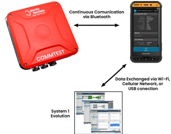
The COMMTEST portable connects via Bluetooth to the handheld, which you can then sync with System 1.
