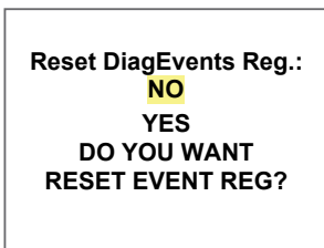
Figure 52: Resetting Diagnostic Events Register
