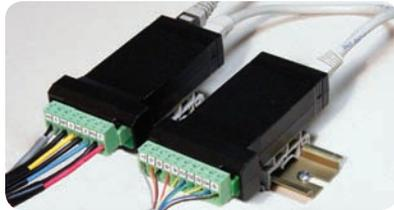
The menu items for these modules do not appear until the module is connected, simplifying the basic menu. Relay and digital I/O modules are shown below with optional DIN rail mounting kit, P/N YPPA1002.
