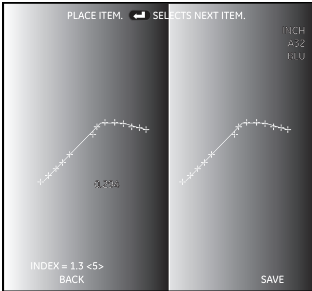
Figure 89: Example of a Depth Measurement
