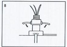
Slide the top in place and push and lock the cam levers into position. Lock cam levers by inserting the stainless steel tie wire through the holes in the ends of the cam levers and twisting together.
