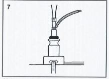
Make sure the sealing grommet is set in the base.
