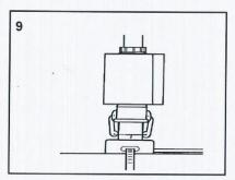
Mount junction box with non-threaded opening for 3/4" conduit, using the sealing gasket and lock ring to hold in place, or use a junction box with a 3/4" inside threaded hub.
