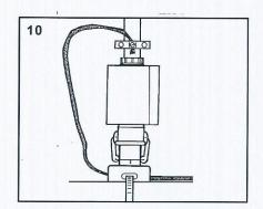
Mount junction box with non-threaded opening for <sup>3</sup>/<sub>4</sub>" conduit, using the sealing gasket and lock ring to hold in place, or use a junction box with a <sup>3</sup>/<sub>4</sub>" inside threaded hub. Ground the braid pigtail to conduit with a clamp (not provided).
