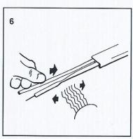
Slide the  $^{1/8}$ " x  $5^{1/2}$ " heat-shrink tubes on the bus wires. Shrink the tubes with heat gun or soft flame torch.
