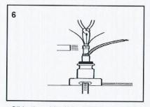
Slide the white 1/2" x 11/2" heat-shrink tube in place over the bus wires and onto the inner jacket. Heat shrink in place. After removing the heat source, and while still hot, pinch the center of the heat-shrink tube between the bus wires with needlenose pliers.
