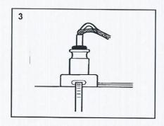
Extend the heater 7'1/2" above the base. Slide the grommet over the heater inserting the grommet in the base. Strip outer jacket 7" from end. Attach the base to the pipe with a pipe strap. (See Heat Trace Stripping Instructions for details.)
