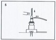
Slide the black  $^{1}/_{8}$ " x  $^{51}/_{2}$ " heat-shrink tubes on the bus wires, and the green/ yellow  $^{1}/_{4}$ " x  $^{51}/_{2}$ " heat- shrink tube on the ground pigtail. Heat shrink, using a heat gun, or soft flame torch, moving the heat source back and forth.
