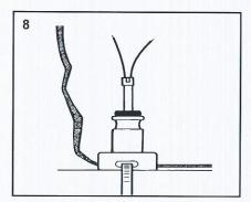
Make sure the sealing grommet is set in the base.
