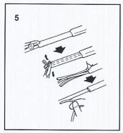
Notch the center core between the conductors and pull the bus wires away from the core for 6". Remove the center core material and any core material on the bus wires. Retwist the bus wires, if needed.
