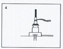
Strip the inner jacket 6" from the end. Strip the bus wires out of the core, following the Heat Trace Stripping Instructions.
