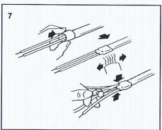
Slide the ½" x 1½" heat-shrink tube over the bus wires and partially over the inner jacket. Heat shrink the tube; while still hot, pinch the center of the heat- shrink tube between the bus wires with needle-nose pliers.
