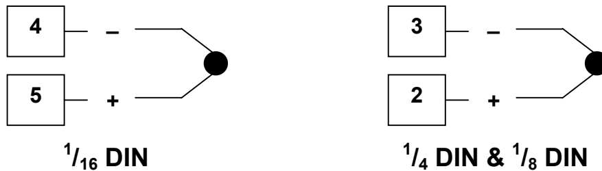
Figure 15. Thermocouple Input Connections
