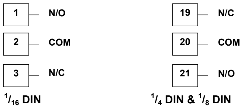
Figure 18. Option Slot 1 – Relay Module
