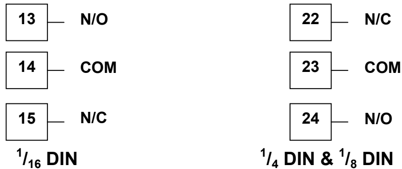
Figure 22. Option Slot 2 - Relay Module
