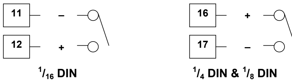
Figure 33. Option Slot A – Digital Input Module
