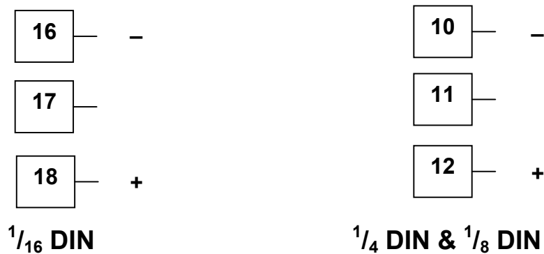
Figure 28. Option Slot 3 - SSR Driver Module
