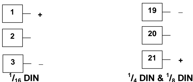
Figure 21. Option Slot 1 - Linear Voltage & mADC Module
