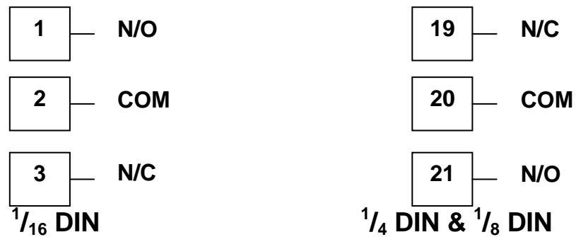
Figure 18. Option Slot 1 – Relay Module
