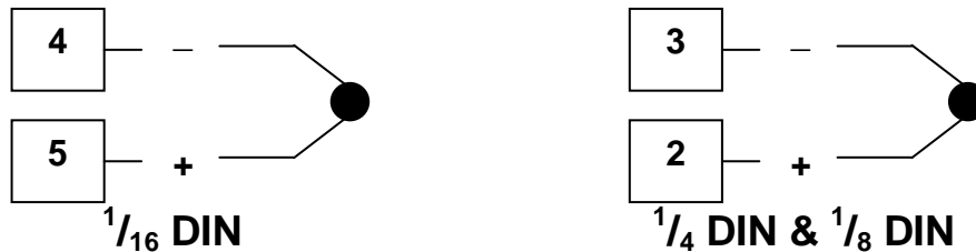
Figure 15. Thermocouple Input Connections
