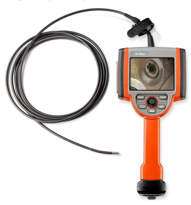
The XL Flex and XL Flex+ VideoProbes provide unmatched image quality and powerful light output to boost probability of detection (POD) and speed up workflow. Rugged durability lowers your maintenance costs. Stereo measurement lets you evaluate defects in depth. And expert support from Baker Hughes gives you peace of mind. All in a lightweight, portable, and easy-to-use device. Now featuring 16GB of memory and an upgraded 5" LCD screen on the XL Flex+.
