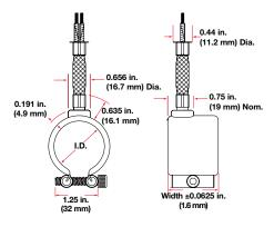
Type E: Loose metal braid encloses two fiberglass leads for good abrasion protection, lead flexibility and wiring convenience. Leads are 2 in. (51 mm) longer than the braid. Shipped with 12 in. (305 mm) leads, unless longer length is specified. To order, specify **Type E** and **length**.
