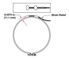
Two fiberglass lead wires exit a single, tightly woven metal braid at a right angle on the expandable construction vs. two sets of leads. The minimum diameter capability is 4 in. (102 mm). Minimum width capability is 1<sup>1</sup>/<sub>2</sub> in. (38 mm). To order, specify **Type SLE** and **length.**
