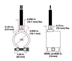
Type F: Loose fiberglass sleeving encloses two fiberglass leads for additional insulation protection where high temperature or minor abrasion is present. Leads are 2 in. (51 mm) longer than the sleeving. To order, specify **Type F** and **length**.
