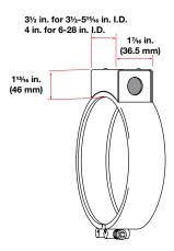
Metallic terminal boxes are available from stock on  $3^{1/2}$  in. inside diameter x  $1^{1/2}$  in. wide (89 mm x 38 mm) or larger heaters. Terminal boxes, which attach directly to the heater, act as a safety feature by covering the terminals. Conduit may be attached to the box through  $^{7/8}$  in. (22 mm) diameter holes in the ends of the box. Two-piece heaters require two boxes. To order, specify **terminal box.**
