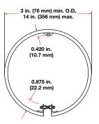
Two fiberglass-insulated lead wires rated to 840°F (450°C) exit a metal braid 180° opposite from gap, Type B outside diameter designed and constructed to mate with inside diameter of cylinders. Maximum width for outside diameter heaters is 6 in. (152 mm). To order, specify **outside diameter and width** of heater.
