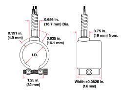
Type H: A flexible steel hose encloses the leads for maximum abrasion protection. Leads are 2 in. (51 mm) longer than hose. Shipped with 12 in. (305 mm) leads, unless longer length is specified. To order, specify **Type H** and **length.**
