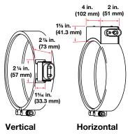
They provide the simplest and safest way to apply power to band heaters. The combination of high-temperature male and female "quick disconnect" plug assemblies eliminates all live exposed terminals and electrical wiring that can be a potential hazard to employees or machine. Maximum 15 amperes at 240VAC, maximum 240V. To order, specify **vertical** or **horizontal** European plug.
