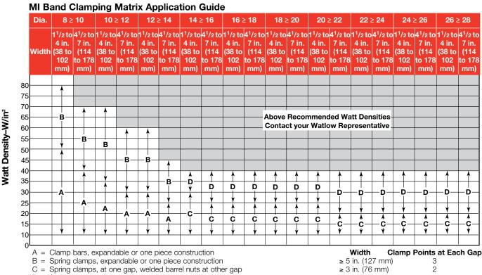
D = Spring clamps, spring clamps at both gaps
