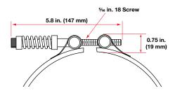
Welded barrel nuts with spring loaded clamping are used to maintain a tight heater fit on large barrels during start-up. This clamping variation is recommended for all MI band heaters greater than 14 in. (356 mm) in diameter and 1½ in. (38 mm) or greater in width. Refer to MI Band Clamping Matrix Application Guide. For smaller diameter heaters, it is an option and must be ordered separately. To order, specify **spring loaded clamping.**
