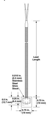
The shim stock thermocouple has low profile and can be placed between components for measurement of surface temperature.
