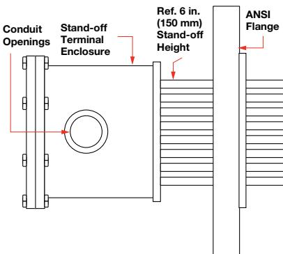
Stand-off terminal enclosures provide an air-insulating barrier between the flange and terminal enclosure by mounting the terminations and wiring away from the flange. Stand-off terminal enclosures are recommended whenever a process operating temperature exceeds 210°F (100°C). This helps minimize terminal enclosure temperatures.
