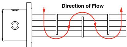
For forced circulation applications, 316 stainless steel baffles can be arranged on the heating element bundle to enhance and/or modify fluid or gas flow for better heat transfer.
