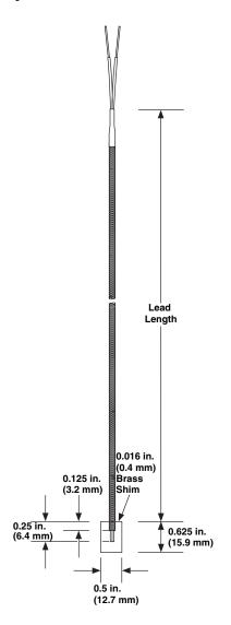
The shim stock thermocouple has low profile and can be placed between components for measurement of surface temperature.
