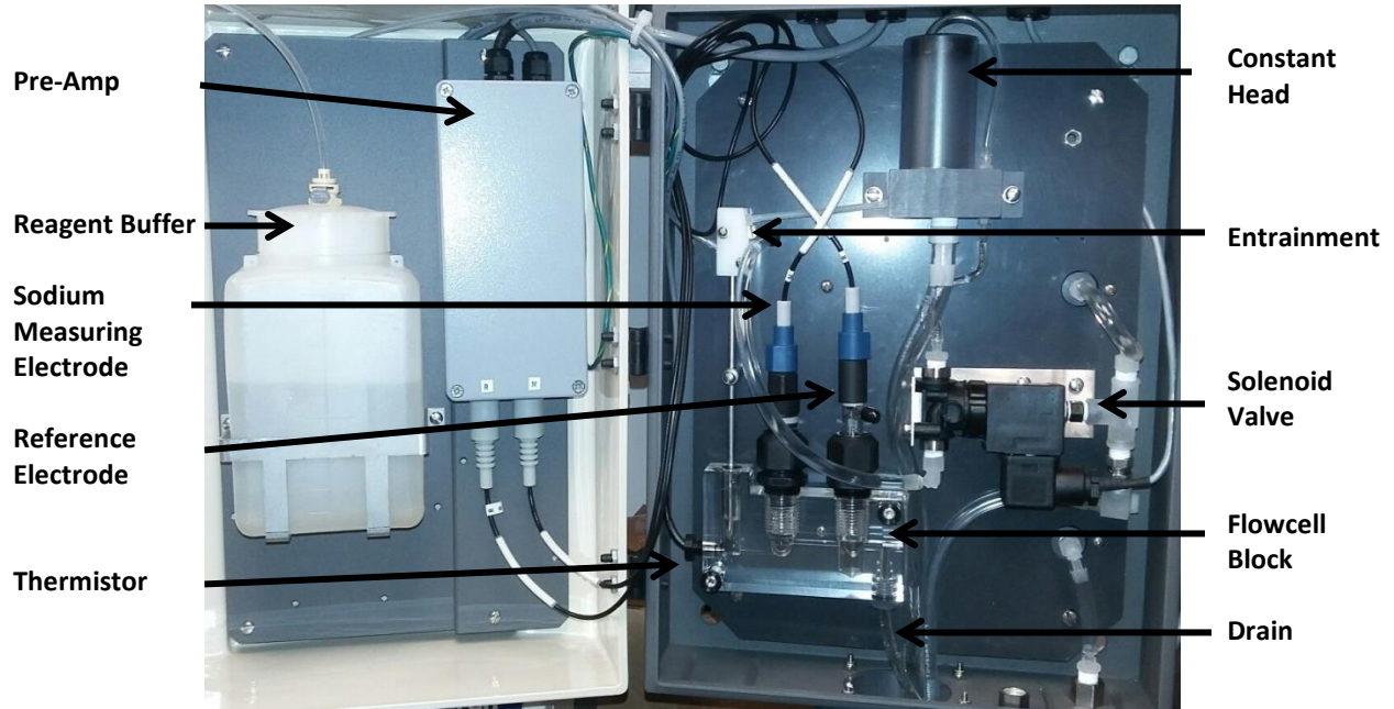
Figure 9 Wet section layout and connections
