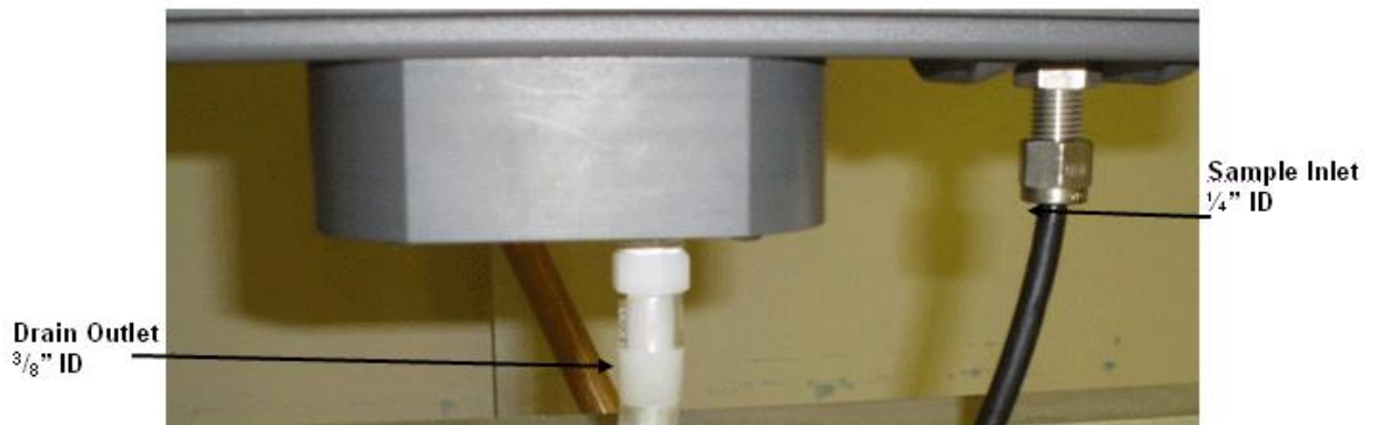
Figure 6 Bottom of the wet section case, with sample inlet and drain connections
