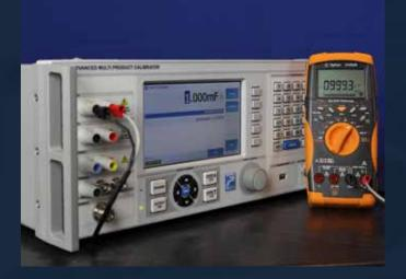
Included in -SYS units, the simulated option provides for resistance calibration between cardinal points and gives a continuous resistance range from 0 Ohms to 1 GOhms, with variable capacitance from 0.95uF through to 100mF.
