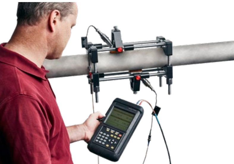
Optional pipe wall thickness gauge
