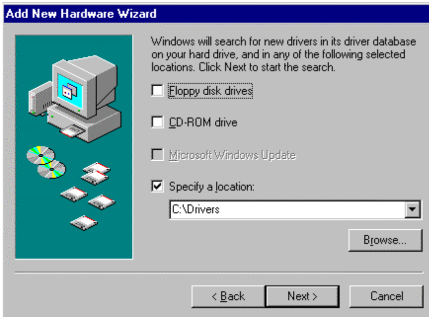
Figure 43. The Add New Hardware Wizard tells you it will search for new drivers, and asks which location(s) you'd like to search. Make sure that only the "Specify a location" box is checked, and click "Next". You will then need to browse to the appropriate file (C:\Drivers).
