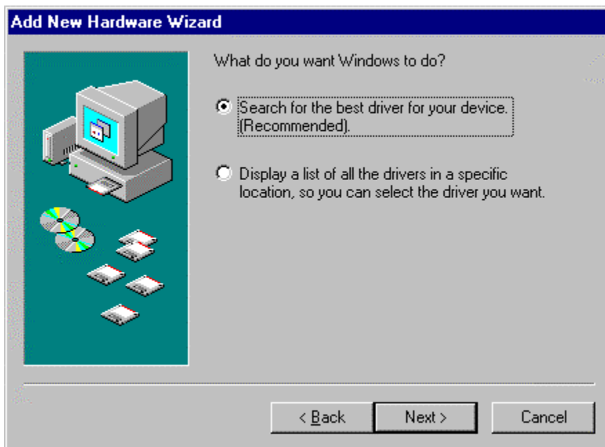
Figure 42. When "asked What do you want Windows to do?", select "Search for the best driver for your device" and click "Next".
