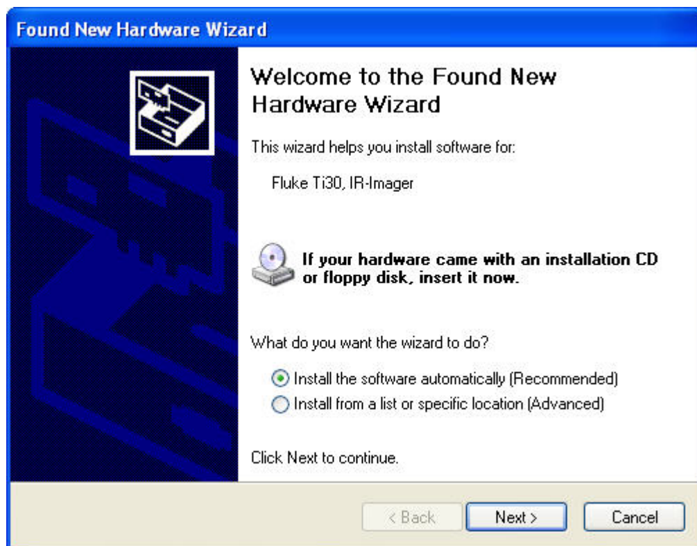
Figure 35. The Found New Hardware Wizard starts. Select "Install the software automatically" and click "Next >".
