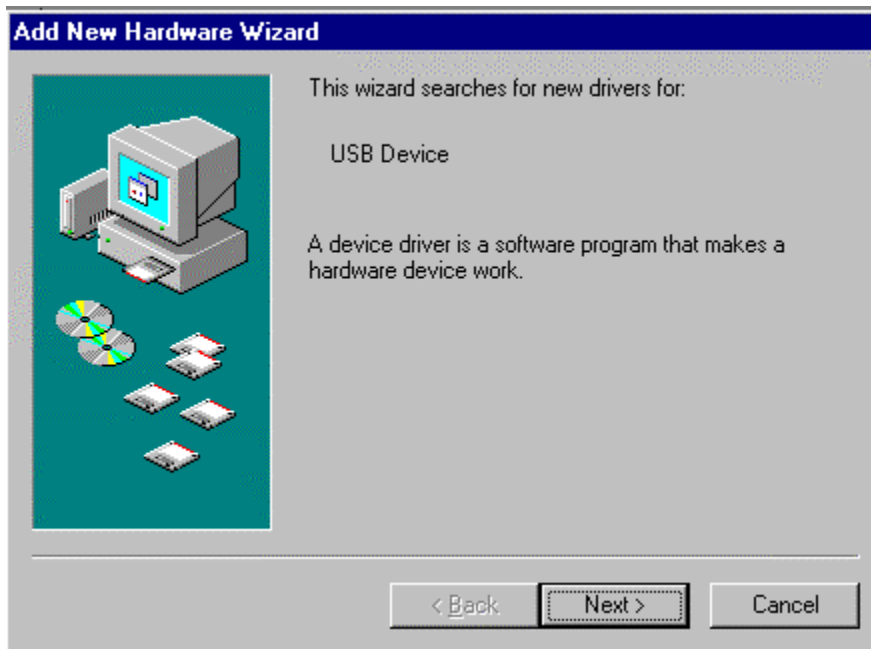
Figure 41. New hardware is detected, and the Add New Hardware Wizard is displayed. Click "Next".
