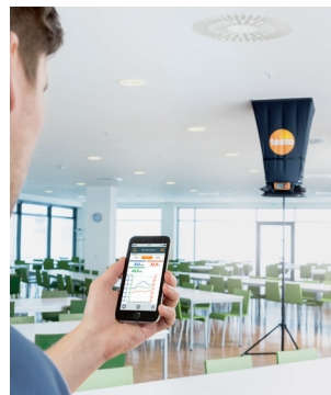
Bluetooth App allows for hands free operation, displaying measurement data on mobile devices and finalizing the measurement report on site.
