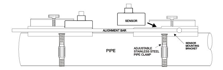
Mount the PC16 Mounting Bracket as illustrated on pipes 0.6" / 15 mm OD or larger. Stainless steel bands are included for mounting on pipes up to 30" / 750 mm OD.
