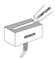
Use the pipe clamp and rail (supplied) as illustrated on previous page or use a loop of electrical tape for temporary mounting. Apply silicon coupling compound #4 to the colored face of the sensor. A bead, similar to toothpaste on a toothbrush, is ideal. Do not overtighten (crush the sensor).
