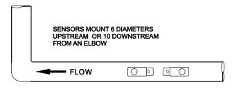
TURBULENCE INCREASING DEVICES: Elbows, flanged connections and tees tend to introduce desirable conditions of an evenly distributed flow profile. Sensor mounting 6 pipe diameters upstream and 10 diameters downstream from these disturbances is generally optimum.
