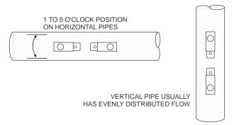
VELOCITY INCREASING DEVICES: Generally the sensors must be mounted away from flow disturbances such as valves, pumps, orifice plates, venturis or pipe inlets and discharges which tend to increase flow velocity. Velocity increasing devices often cause cavitation, or rapid release of gas bubbles, and readings both up and downstream may be intermittent or inaccurate. As a guideline, mount the sensor at least 20 diameters upstream or 30 diameters downstream from velocity increasing devices.
