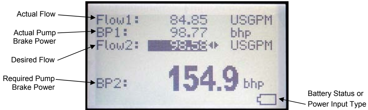
Figure 13: Pump Law Brake Power Screen
