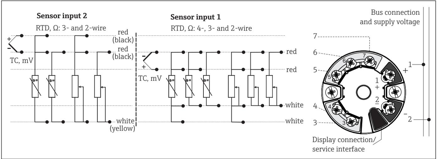
3 Assignment of terminal connections for head transmitter
